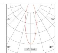
Light Distribution Auro Tube 60 Profile Systems Light Beam Talbe Colour Temperature 2700/3000/3500/4000K Colour Rendition Index CRI 90 Optics PC Beam Angle 108D Installation method Suspension Connected Load 34W/m Luminous Flux Of The Luminaire 4618lm Luminaire Efficacy 117.68lm/W Colour Deviation SDCM<5 Light Source LED LED Type SMD **Dimming Method** On/Off/0-10V/ Dali Cover Material Aluminum Body Material Aluminum IP Rating IP20 Housing Colour Sandy White/ Sandy Black Weight
